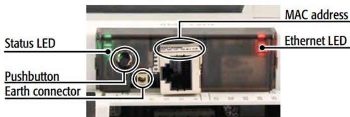
Figure 17-15: BACNET TCP/IP board detail.
