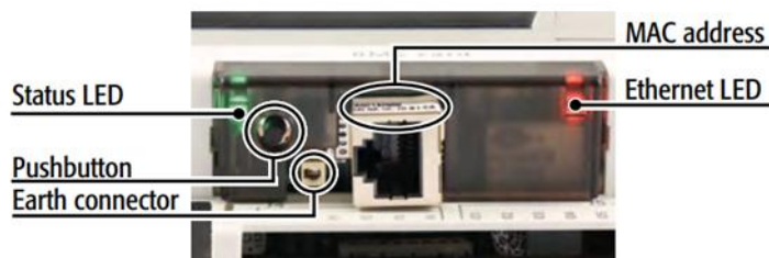
Figure 11-4: BACNET TCP/IP board detail.
