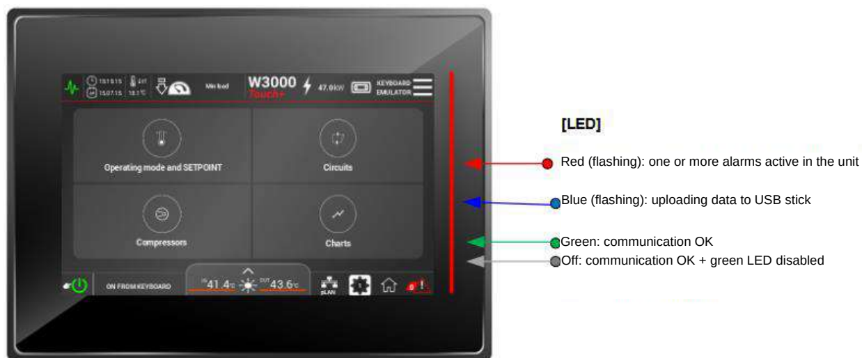
Figure 2-8: Explanation of the various elements of the W3000+ touch keyboard with 7" screen.
