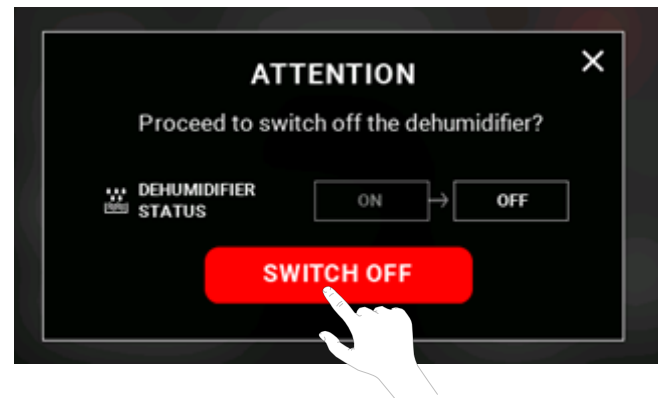
Figure 16-43: dehumidifier switching off screen.
