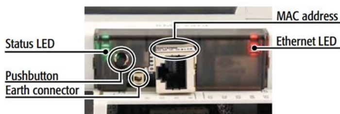
Figure 17-22: pCOweb board detail.
