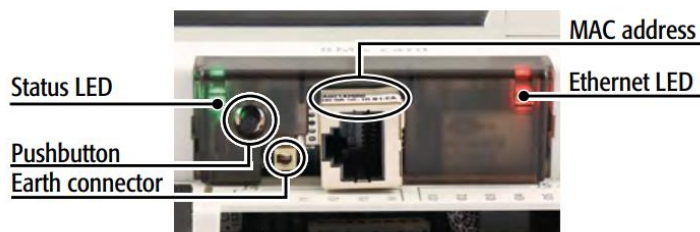
Figure 17-5: MODBUS over IP board detail.
