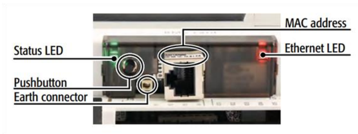
Figure 9-4: MODBUS over IP board detail.
