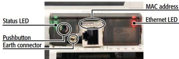
Figure 16-3: pCOweb board detail.
