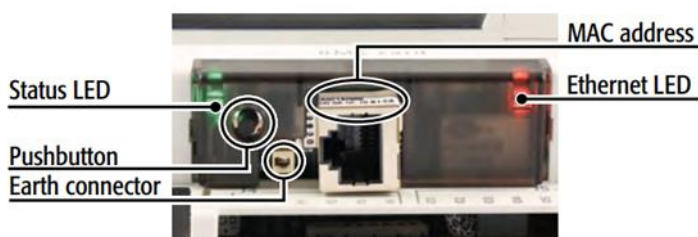
Figure 11-4: BACNET TCP/IP board detail.
