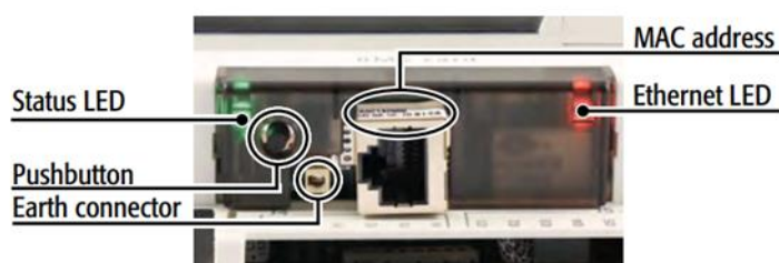
Figure 17-15: BACNET TCP/IP board detail.
